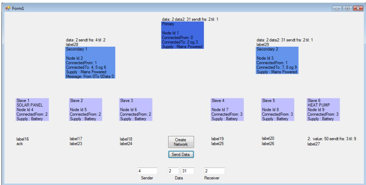
**Figure 7.3:** Information from a solar panel is gathered on the left side subsystem and on the behavior of the value it reduces heat pump activity.
